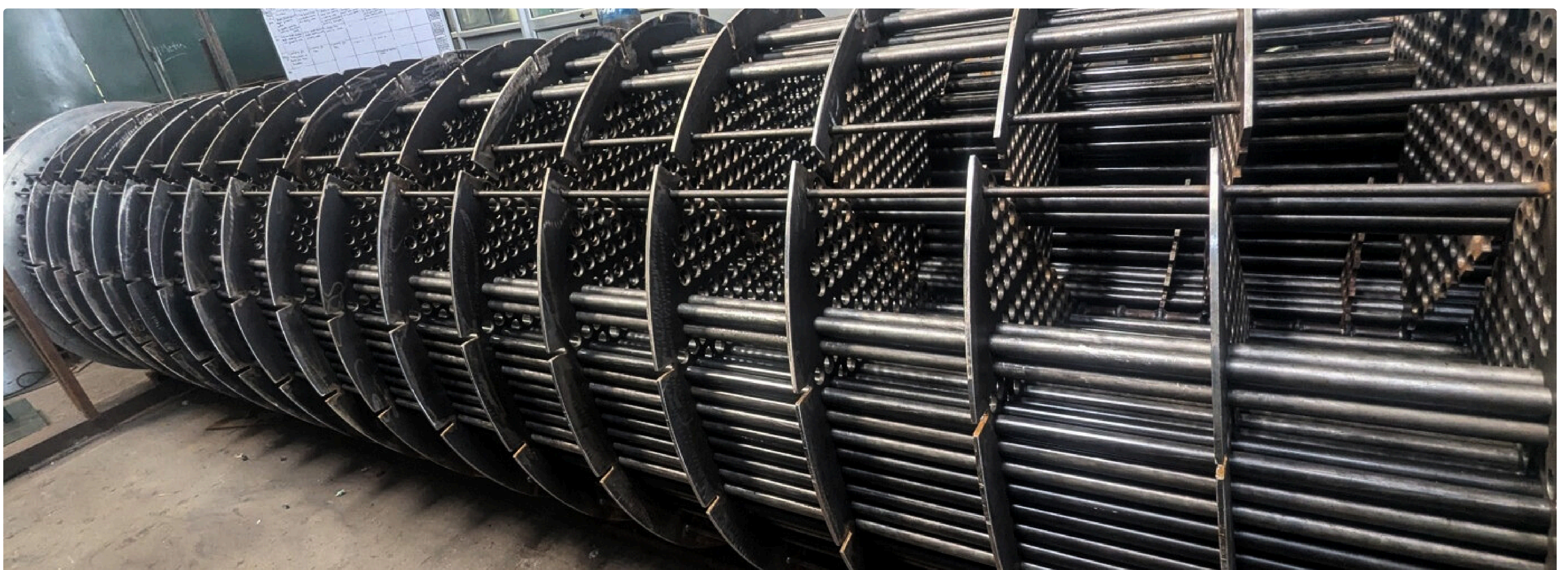
Helical Tube Bundle for MRPL Mangalore
