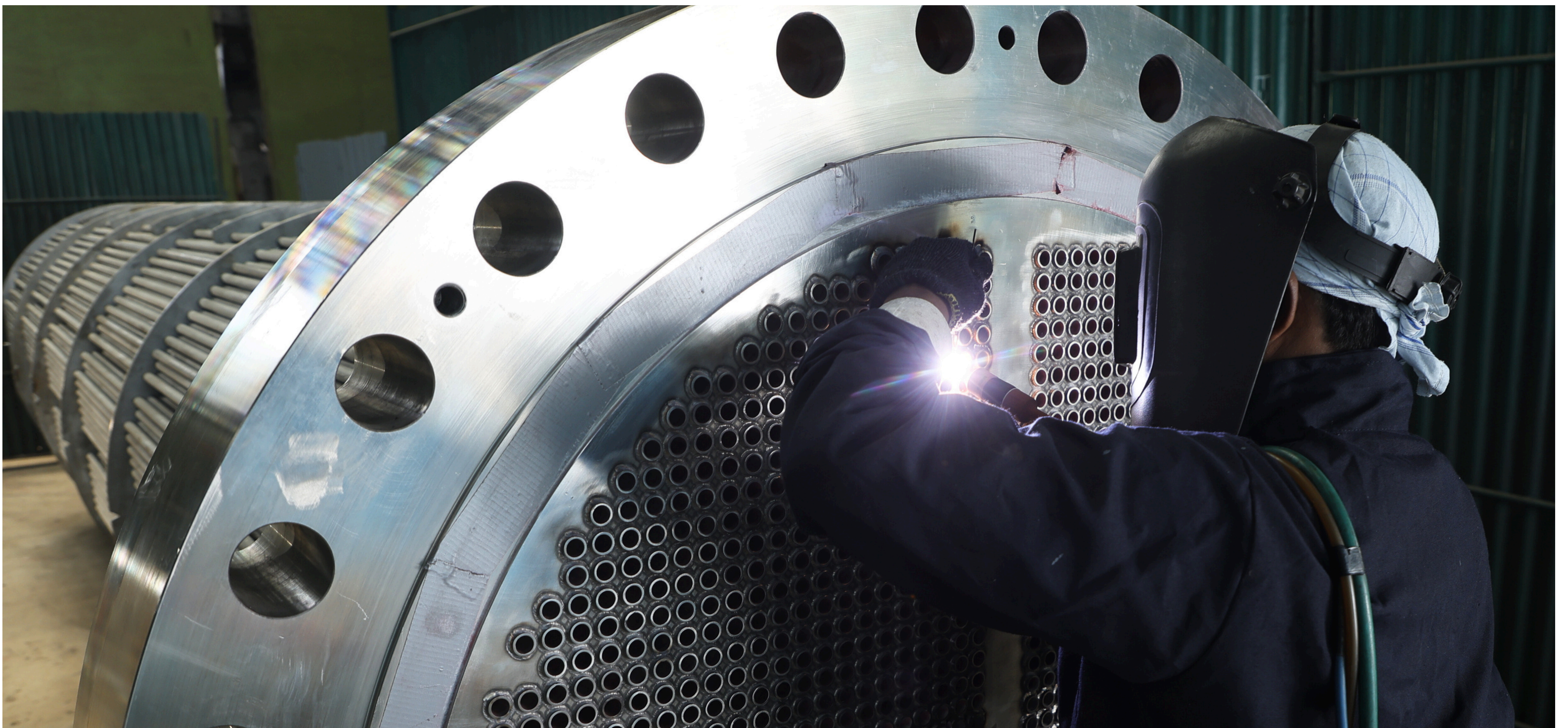
SS347 U-Tube Bundle for HPCL Mumbai Refinery
